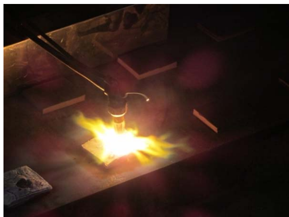
Figure 2. Photograph of the oxyacetylene ablation process. [Color figure can be viewed in the online issue, which is available at wileyonlinelibrary.com .]
